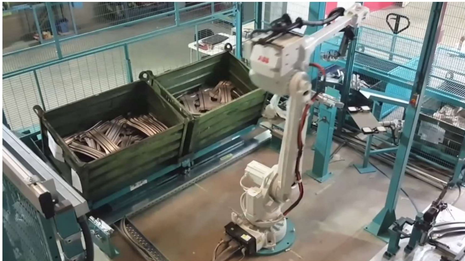
Kilde: Robotic Bin Picking on stamped parts with ABB robot in production at GEDIA - VISIONERF
