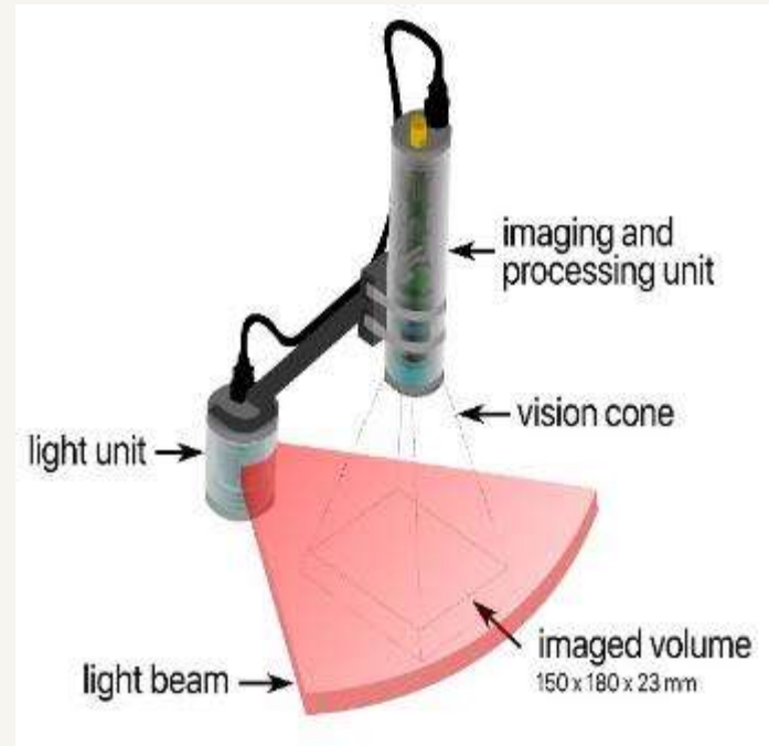
Fig. 2 The Underwater Vision Profiler version 6 (UVP 6). Drawing based on Picheral et al. (2021)
